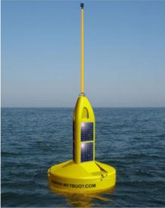
Weather Buoy / Data Buoy / Oceanographic Buoy operated by the MDS
